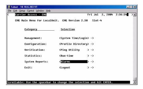
This Window provides a listing of any Alarms that have occurred on the Router. Each Alarm is listed separately and the Count field will display a value of 1. See *Alarms on page 9-4* for more information regarding this feature.
